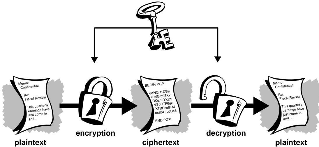
**Figure 1-2. Conventional encryption**
